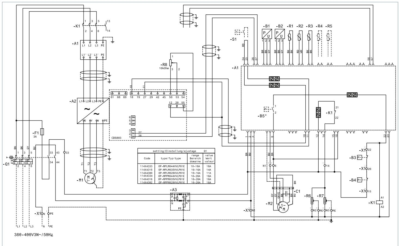
A1 : EMC/RFI Filter (Compressor)
